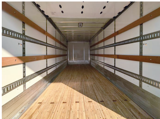
Crossmembers are hot-dipped galvanized and support the standard 1-1/8" laminated oak floor.
