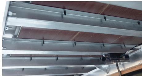
Crossmembers are hot-dipped galvanized and support the standard 1-1/8" laminated oak floor.
