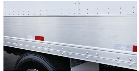
Extended bottom rail and composite side panels provide greater durability.
