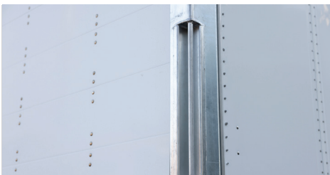
The inset grab handles are protected against impact damage.
